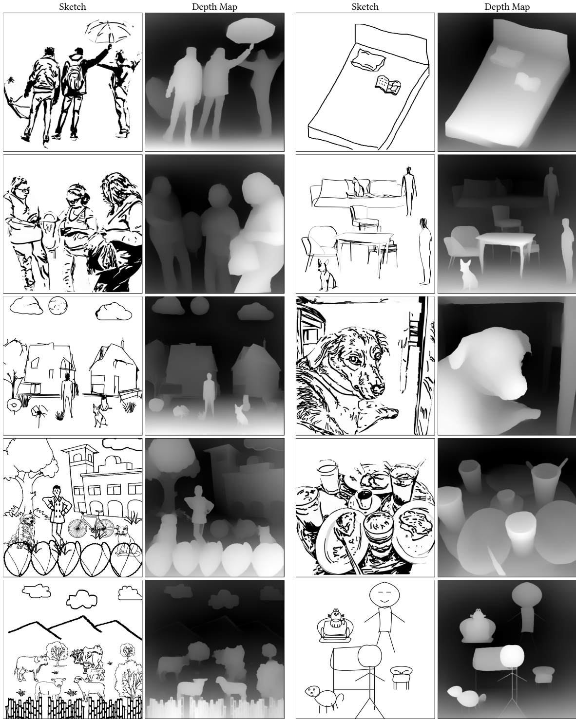
Fig. 15. Sketch and corresponding DepthAnythingV2 [2024] depth map pairs. We show qualitative results on sketch depth maps of scenes across datasets, demonstrating the reasonable performance of this depth estimator directly on sketches. The model generalizes surprisingly well across a wide spectrum of sketch styles, from highly abstract and symbolic representations to more detailed and realistic ones. Despite the lack of color or shading cues, the predicted depth maps often capture overall scene layout and object ordering effectively.
